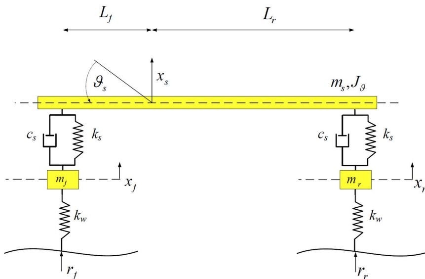
Fig. 2. A kinematic model of a passive suspension [3]
