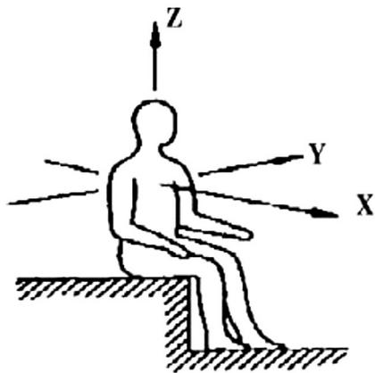
Fig. 1. The system of coordinates usable for assessing the vibrations that affect a human body [5]
