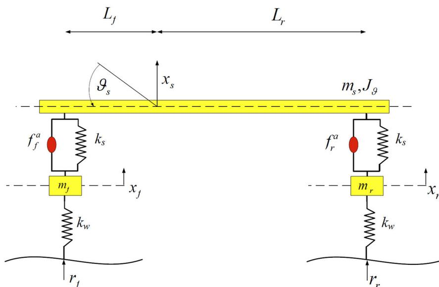
Fig. 3. A kinematic model of an active suspension [3]
