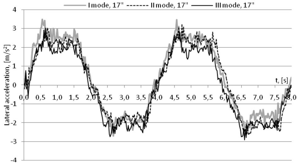
Fig. 7. Fluctuations of the lateral acceleration for different heights of the vehicle body
