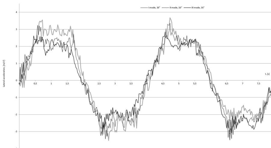
Fig. 6. Fluctuations of the lateral acceleration for different heights of the vehicle body
